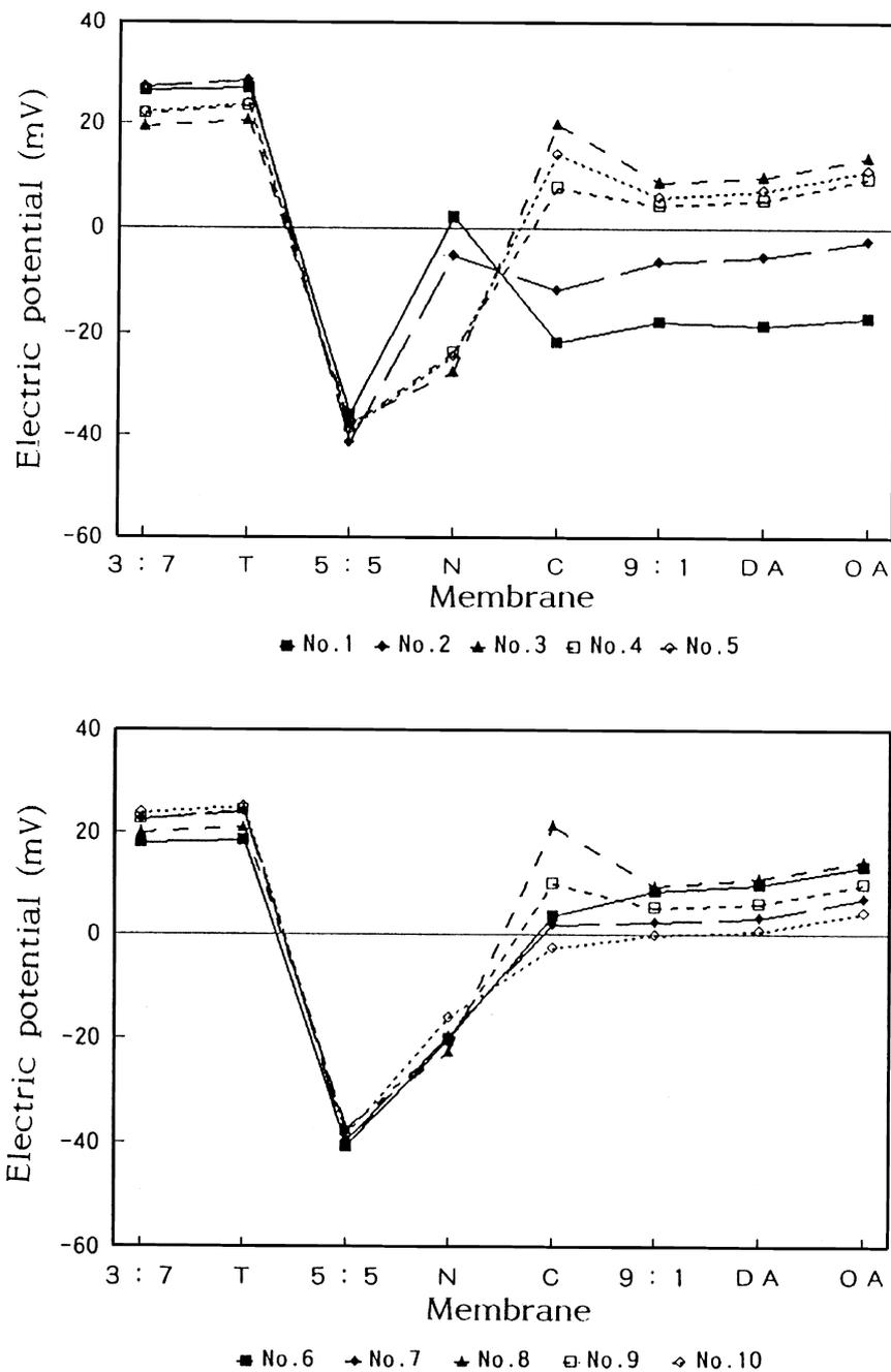
Fig. 2. Response of multichannel electrode to water quality in Onga river. No. 1: the source of the river, No. 10: the mouth of the river.
