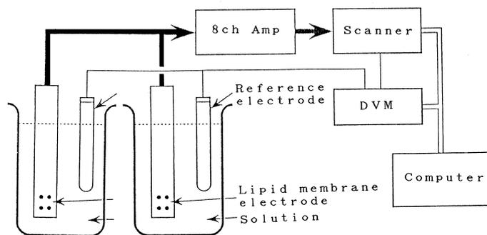
Fig. 1. Schematic diagram of multichannel electrode system.
