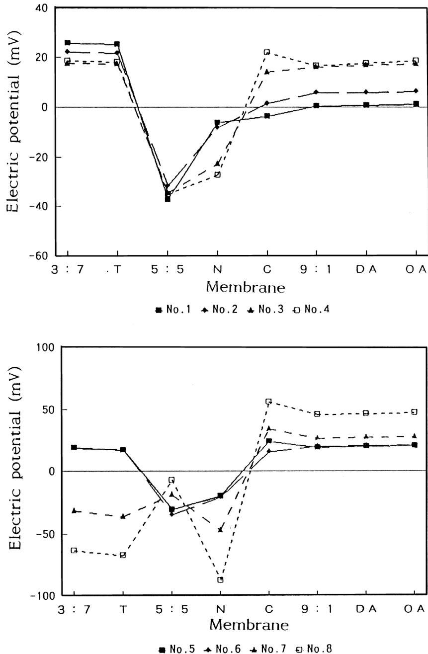
Fig. 3. Response of multichannel electrode to water quality in Murasaki river. No. 1: the source of the river (Musubutci dam), No. 8: the mouth of the river.
